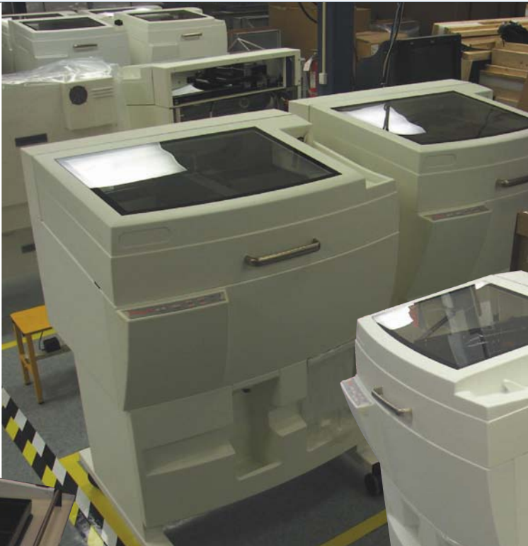
These photos above, below and to the left and right show Z Corp.'s 3-D printers in various stages of production. Each phase of assembly is done at a unique work cell with dedicated personnel. Additional employee training and Kanban replenishment strategies have been key in managing work flow.
