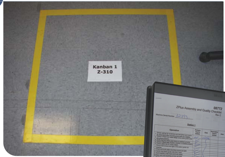
(left) Each work cell at Z Corp. is set-up ahead of time with the proper tools and components. Additionally, work cell postings (above) and documentation (right) keep employees accountable in executing replenishment strategies.
